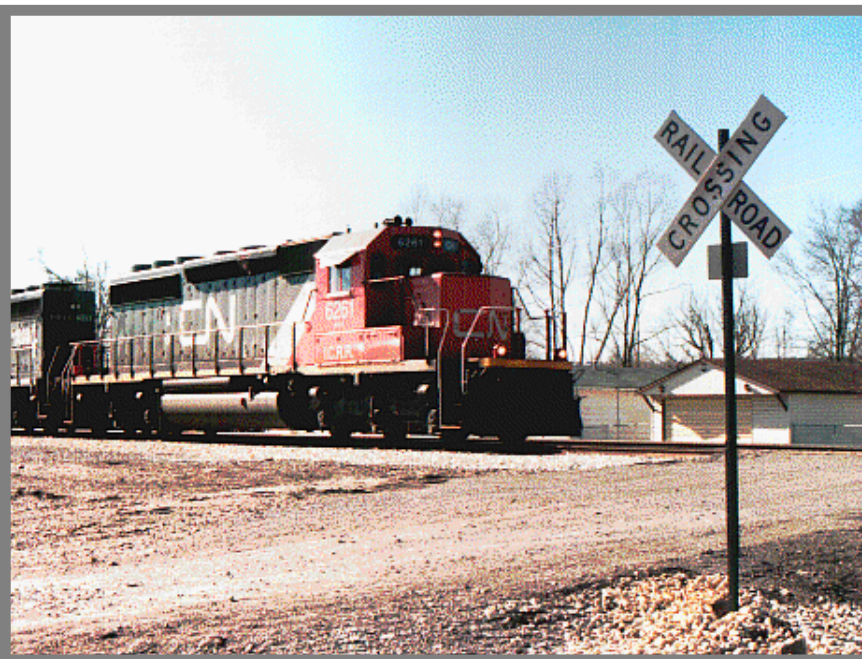
CN/IC SD40-3 6261 on n/b empty coal train at Big Bay, Illinois. January 7, 2000. This unit is exx BN 6753, ex IC 6150 and was outshopped as an SD40-3 on 12/07/99.
